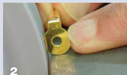
2 Grinding the flat washer. Keep it cool, and always hold it in the trailing position as shown. Make sure your toolrest is as close as possible to the rotating wheel.
